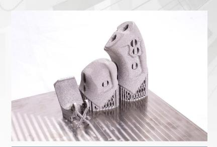
Objects are created from 3D data, layer upon layer – thus adding not subtracting and wasting raw materials as in conventional parts manufacture.
