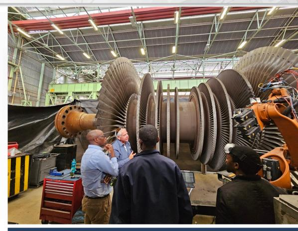
Both laser cladding and welding processing use robotics to deliver light and deposition material to working surfaces; A mobile unit can perform the work at client site.
